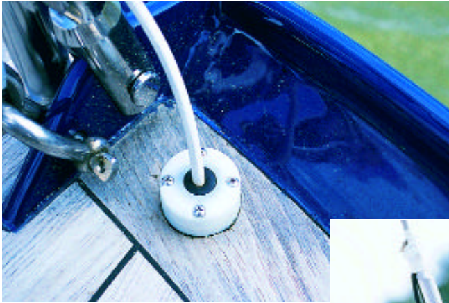
Above, GTO cable will suffer if repeatedly stepped on. Use a plastic and rubber through-deck fitting that prevents a sharp metal edge to make contact with the cable. Right, swaged backstay insulators require the services of a rigger for installation.
