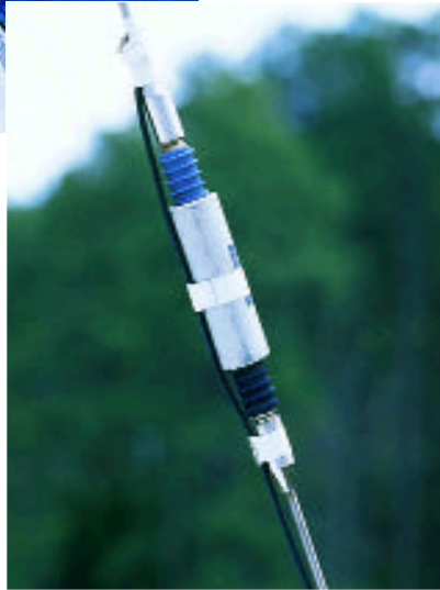
Above, GTO cable will suffer if repeatedly stepped on. Use a plastic and rubber through-deck fitting that prevents a sharp metal edge to make contact with the cable. Right, swaged backstay insulators require the services of a rigger for installation.
