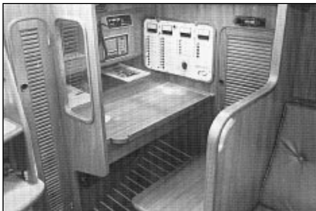
The nav station is compact, but workable. Note the superb electrical panel, protection from spray coming through the companionway, and wet locker next to the companionway steps.
